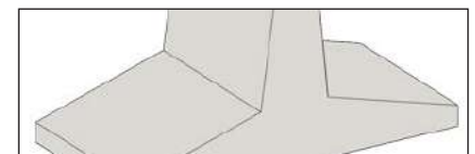
A slab retaining wall.
